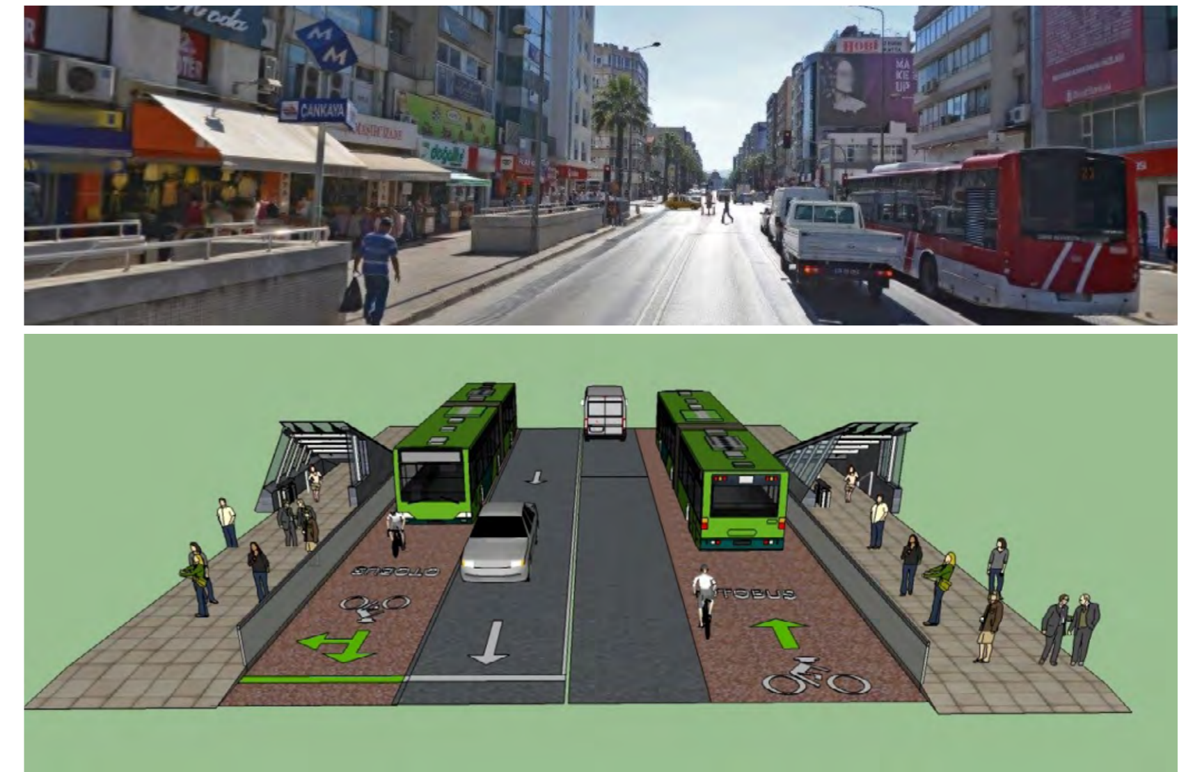
Figure 17 | Conceptual Design Belonging to the Shared Bus-Bike Lane Application for the Road Platform on Fevzi Paşa Avenue Near the Çankaya Intersection
